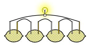
A way of making this experiment more impressive is to use a set of lemons in series using crocodile clips to trickle charge a capacitor. Then discharge this through an LED to give a flash of light like the camera flash.
