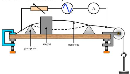
Vary the tension and the length until the wire vibrates strongly, i.e. a resonance condition has been found. Record the length (L) and the tension (T) for series of pairs of values. Measure the mass per unit length (m) of the wire.
