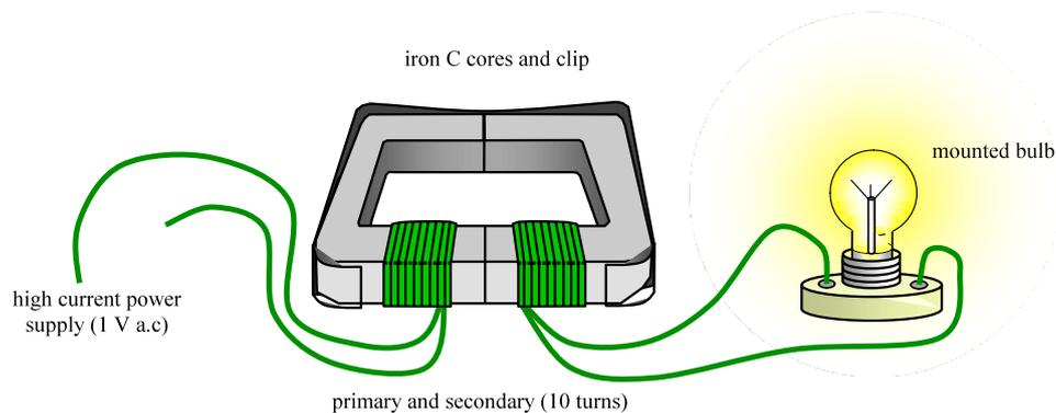
Connect the apparatus as shown with one coil fixed to the 1 V AC output of the power supply. Record what happens to the bulb. Now try reducing the number of turns on the secondary, and then reducing the number of turns on the primary. What happens to the bulb in each case? Describe and explain what happens if the C cores are slightly separated. Record all readings and observations on the Worksheet.
