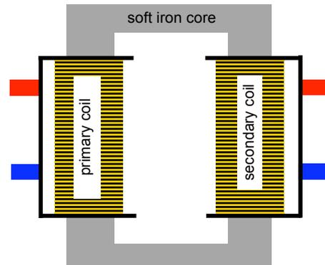
A transformer consists of two coils - the primary coil and the secondary coil both wound on a soft iron core as you can see from the diagram. If an ac. voltage is applied to the primary coil then this will produce a changing magnetic field in the iron core. This then induces an alternating voltage in the secondary coil.
